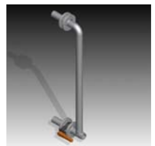
Overflow and drain
